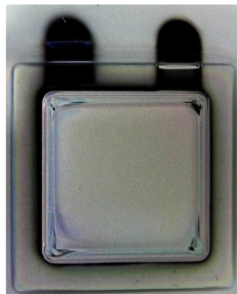
Figure 2: Photographic picture of 250 \mu Ah Stereax M250 solid state battery.
