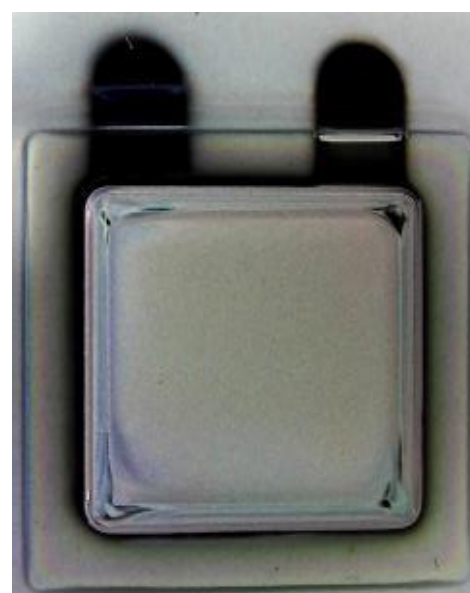
Figure 2: Photographic picture of 250 \mu Ah Stereax® M250 solid state battery.
