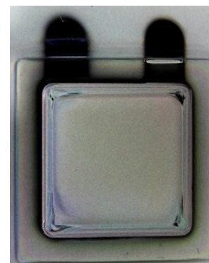
Figure 2: Photographic picture of 250 μAh Stereax M250 solid state battery.
