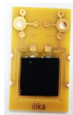
Stereax P180 solid state batteries on evaluation PCB
