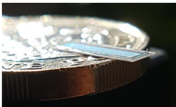
Miniature Stereax solid state battery basic unit cell
