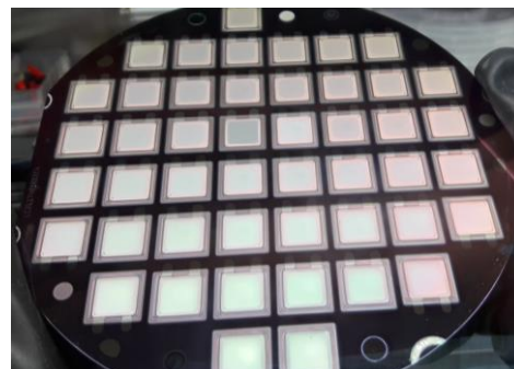
Stereax P180 solid state batteries deposited on 6" wafer
